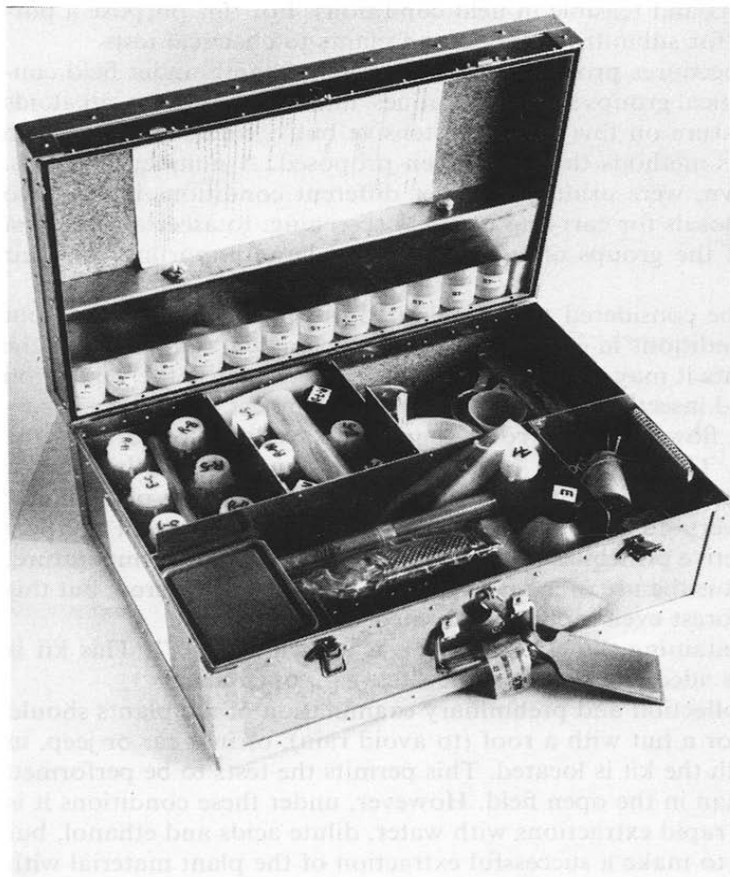
Fig. 1. Transportable kit for field chemical screening of plants.
